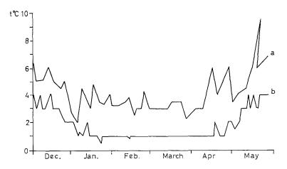
Fig. 3: Temperature records from the main culture tank (a) and the first level of the laboratory building (b), Marine Sciences Research Laboratory, Logy Bay, Newfoundland. December 1968 to May 1969
