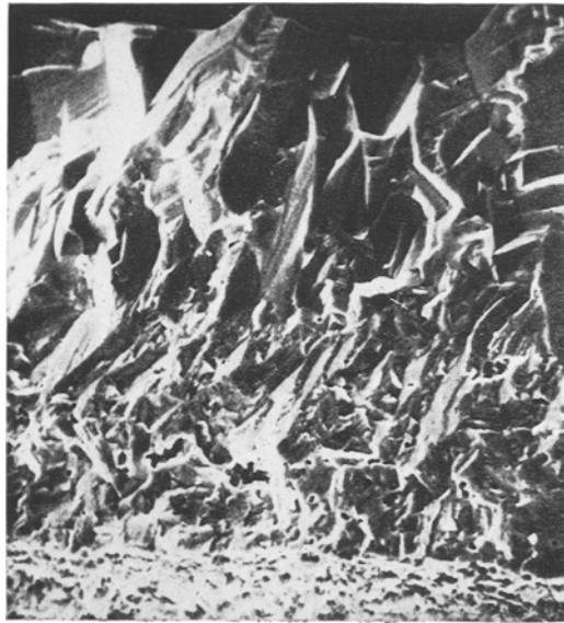
Fig. 3b. Scanning electron micrograph of fractured scale section on Ni-2%Cr oxidized at 1200°C (magnification \times 1000 ). (Courtesy of J. E. Castle and I.I.T. Research Institute Symposium.)
