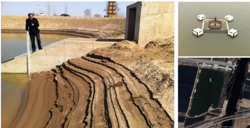
Fig. 2.6 Infiltration basin in Guantao County with water depth gauge (left) and floating evaporation pan (upper right) to measure evaporative losses. A satellite image (bottom right) shows the extent of the infiltration pond, which is called “Moon Lake”
