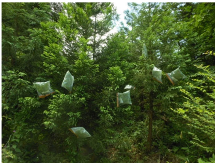
Fig. 13.5 Trapping transpiration water from the leaves of young Cryptomeria japonica using plastic bags in June 2013
