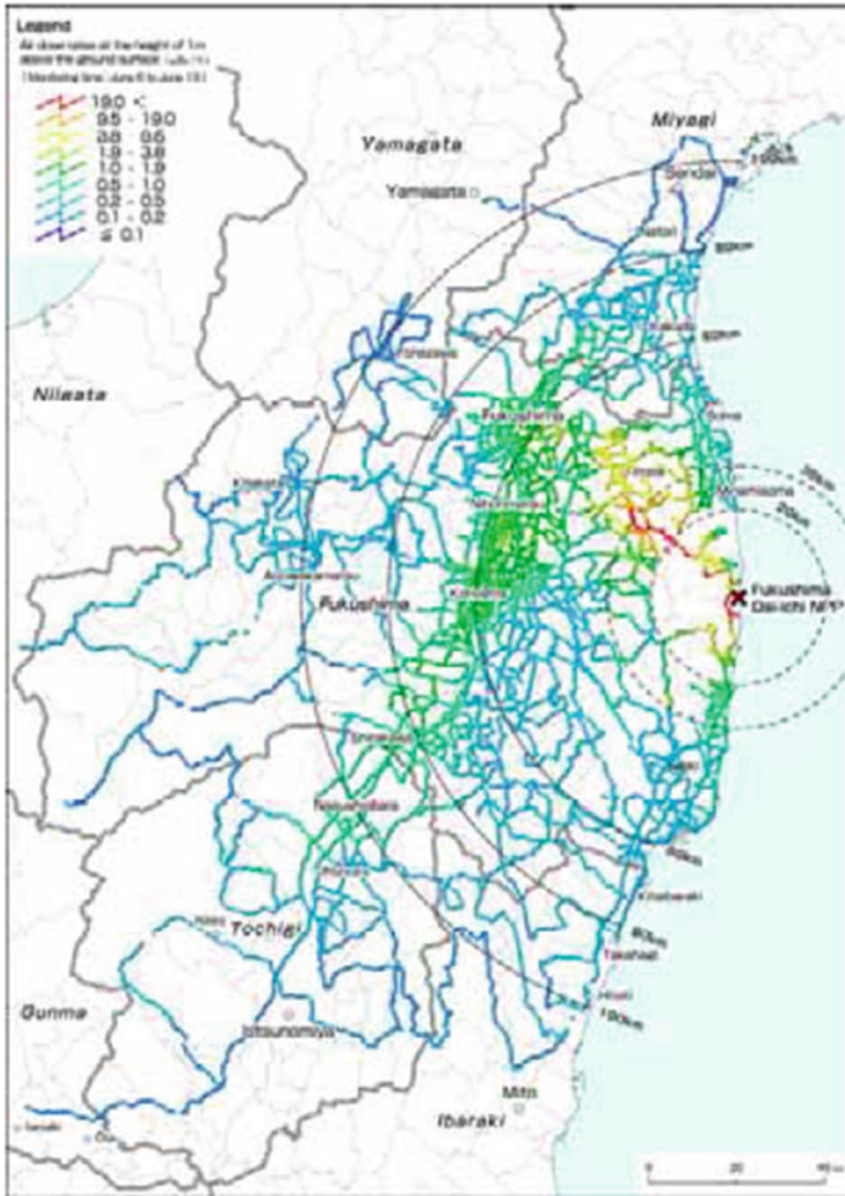
Fig. 1.2 Distribution map of ambient dose rates based on continuous measurement results from vehicle-borne survey [3]
