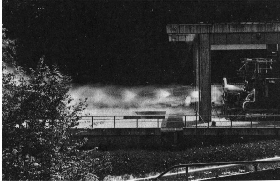
Fig. 15 DLR Lampoldshausen, ARIANE V project - test run of 100 kN combustion chamber on P3.2 test stand
