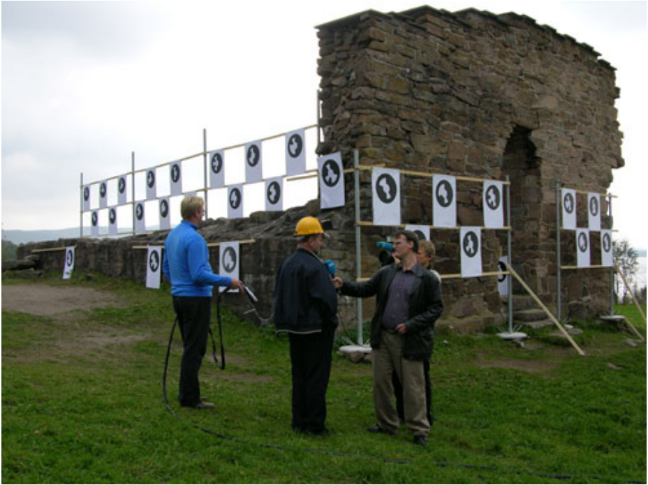
Fig. 1. AR markers placed on the ruin of the Margareta Church in Maridalen, Oslo, Norway
