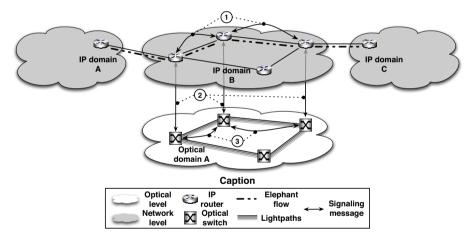
**Fig. 1.** Self-management of lightpaths in hybrid optical and packet networks: in step 1, the elephant flows are identified; in step 2 the optical switches are informed about the decision to move a flow; and in step 3, the optical switches establish the lightpath.
