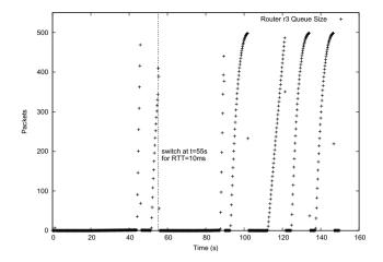
Fig. 7. Router r3 Queue Size for 10Gbps case with RTT = 10ms
