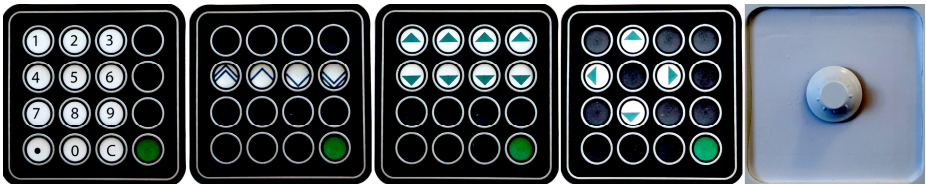
Fig. 1. The different configurations of interfaces used in our setup. From left to right (a) Number pad (b) Chevrons (c) Up-down (d) Five key (e) Dial
