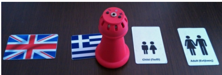
Fig. 2. Setting the user’s profile by “listening to” appropriately marked RFID tags
