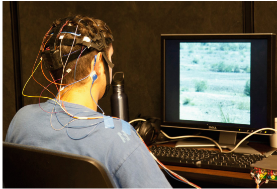
Fig. 5. Photograph of one subject in the test environment. The Cognionics 32-channel dry headset was placed on a subject. Standard wet adhesive electrodes, on top of abraded scalp, were placed adjacent to select dry electrodes and connected to a g.tec amplifier for simultaneous recordings.
