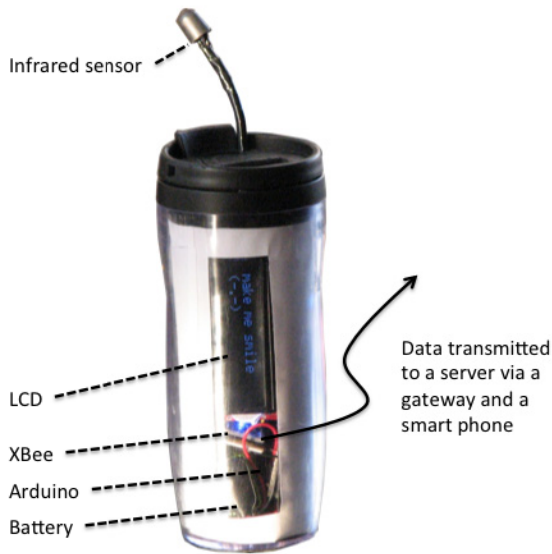
Fig. 2. Prototype “contextual sensor”
