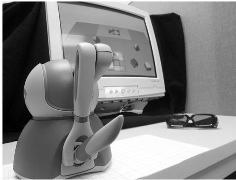
Fig. 1. VR-BD training apparatus including PHANTOM Omni and NVIDIA 3D Vision kit
