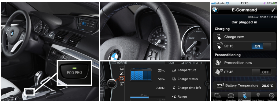
Fig. 2. BMW ActiveE interior (Fotocredit: BMW Group): Location of the ECO PRO button (left), instrument cluster and central display with vehicle energy information. Smartphone display of vehicle energy functions (right)
