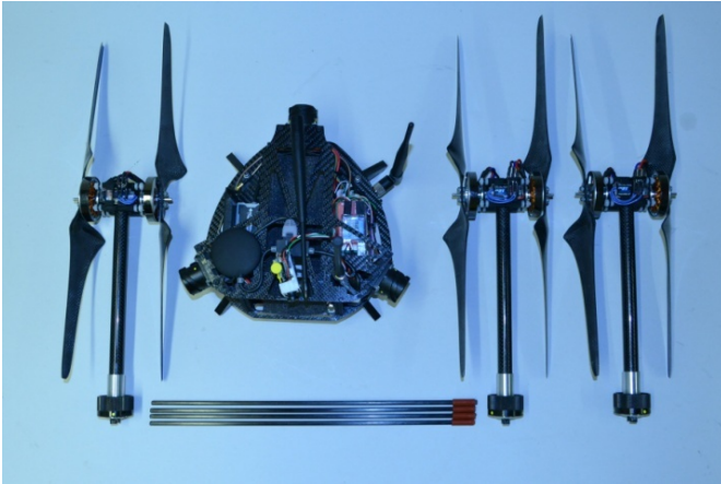
Fig. 4. HALO UAV Showing Detachable Elements
