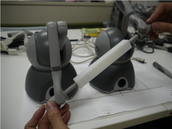
Fig. 2. Two haptic devices connected by connecting bar
