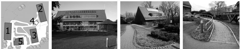
Fig. 1. Windmühle Seifhennersdorf – from the left: situation (site plan), large hotel, small hotel, adjusted terrain – wheelchair slope and bridge (on the plan: 1 – service building: restaurants, library, meeting halls; 2– large hotel with rooms for the disabled; 3 – small hotel, with rooms for the disabled, 4 – elevator leading to the lower level with workshops 5 – regional house – reception, meeting rooms [Elaborated on the basis of evacuation plans [13]).
