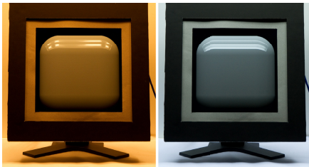
Fig. 8. Simulating gloss. Note that the colors and patterns of the glossy highlights are correct with respect to the different light booth luminaires
