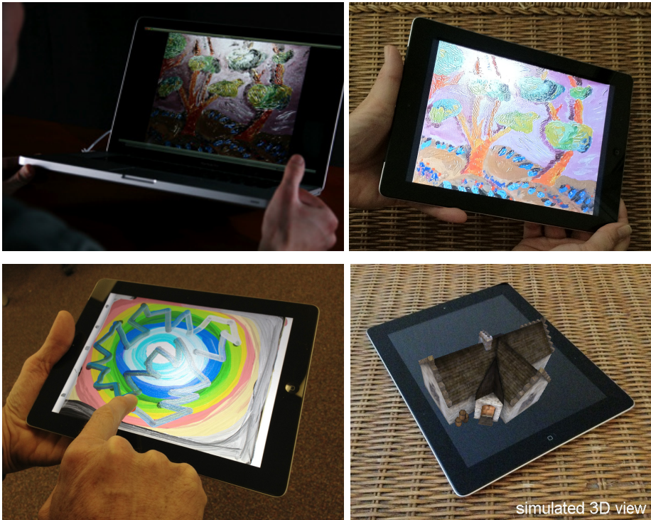
Fig. 1. Tangible imaging systems (left to right, top to bottom): The first generation tang iBook system developed using an off-the-shelf laptop computer; the tangiView system implemented on a tablet device; the tangiPaint application that allows direct creation of and interaction with rich digital paintings; the phantoView system that allows tangible interaction with three-dimensional object models
