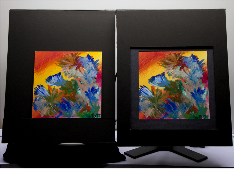
Fig. 10. Simulating surface appearance. The real painting is on the left the image produced by the system is on the right. Note the realism of the color, gloss, and texture components. As noted in the text, the image also meets the responsiveness and situatedness requirements of tangible imaging systems.
