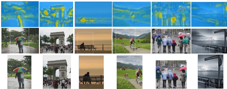
Fig. 4. Visual comparison of still pictures for the seam carving and dynamic reframing schemes. Top row is the computed saliency heat maps (the reddish pixels are salient, the blue ones are not). Second row is the original picture with the cropping window in white. Third row is the resulting cropped picture.
