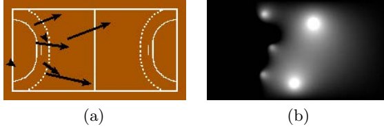
Fig. 3. Generating a motion-information image using frame differencing. (a) Team players movements. (b) The motion-information image.
