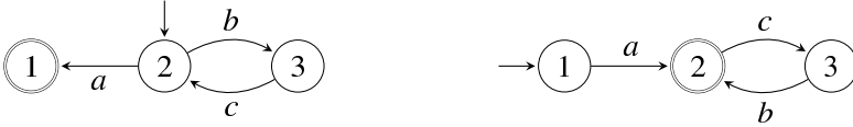
Fig. 6. SPA G (left), and DFA G^R for the reversal of the language L(G) (right); projection P : \{a, b, c\}^* \rightarrow \{a, c\}^*
