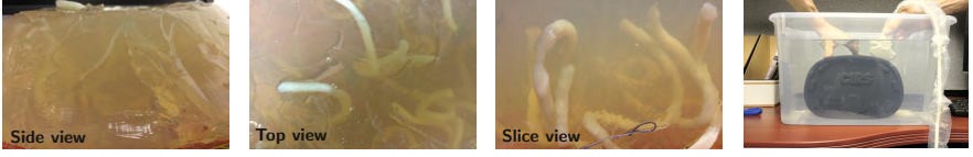
Fig. 2. Illustration of the noodle phantom , made of gelatine and Soba noodles (left three images) and an abdominal CIRS phantom mounted in a water tank (right)
