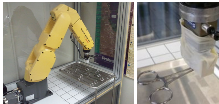
Fig. 4. (a) FANUC Robot (b) Latex-encased magnetic gripper
