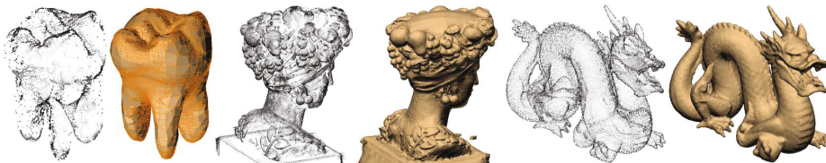
Fig. 1. We have developed a new method of reconstructing high resolution watertight surfaces from oriented points which is particularly good at extrapolating under-sampled areas, missing and irregularly sampled data [7]
