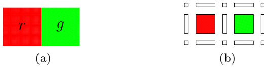
Fig. 1. (a) A digital image \lambda in \mathbb{Z}^2 with 2 labels r (red), g (green) and a background (not depicted). (b) The embedding of the image \lambda in \mathbb{F}^2 , the space of cubical 2-complexes, obtained by applying the following membership rule: the label of a face is the infimum of the labels of the surrounding facets in the poset (2^{\{r,g\}}, \subseteq) . We have proved in [10] that this embedding preserves the connected components and the fundamental groups of the object and its complement when a binary digital image is interpreted with the (2n, 3^n - 1) -adjacency pair. But, if we identify the two labels, that is if we consider a coarser partition of the space, the topology is not the same on these two images (we have one component on the left and two components on the right).
