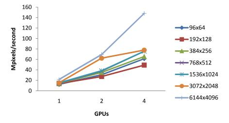
Fig. 7. Mpixels/sec executed by both kernels (no memory transfers accounted)
