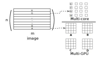
Fig. 3. Image divided in 4 GPUs and 4 cores
