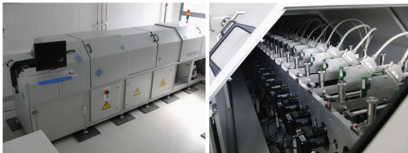
Fig. 7.8 (a) The peptide laser printer. (b) Horizontal setup of the 24 development units (printing cartridges) assembled in a row
