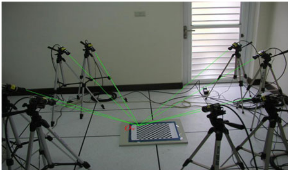
Fig. 3. Part of the multi-view video capturing configuration
