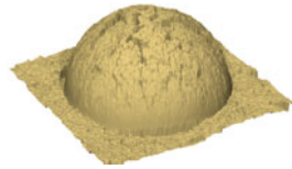
Fig. 3. Output of Fraile-Hancock’s integrator [5] applied to the gradient data of figure 1 with noise added
