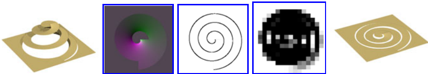
Fig. 5. A height map, its gradient map, weight map (256x256 and 16x16 scale) and the integrator's output [16] after 200 iterations
