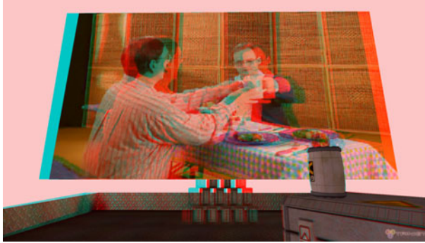
Fig. 2. The scene illustrates the three different depth settings and respective parallax differences caused by unadjusted MSVR: Note that the occlusion mesh's parallax causes a black border and that due to the differences between scene and video parallaxes it becomes difficult to fuse the images.
