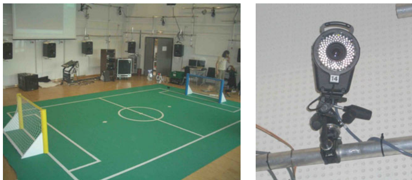
Fig. 1. The experimental setup for the data recording. The left image shows the RoboCup Standard Platform League field within motion capturing system. The right image shows one of the 15 cameras of the body motion tracking system. The LEDs at the front of the camera provide pulsed infra-red light allowing capturing under day light conditions.
