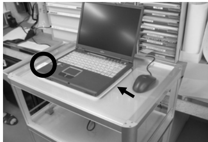
Fig. 3. A wireless LAN terminal at SUH (circle, wireless LAN card; arrow, a vibration-absorbing mat)
