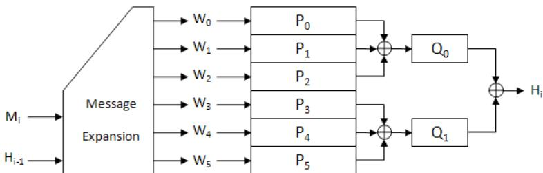
**Fig. 1.** The compression function of LANE
