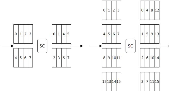
**Fig. 3.** SwapColumns operations used in LANE-256 and LANE-512
