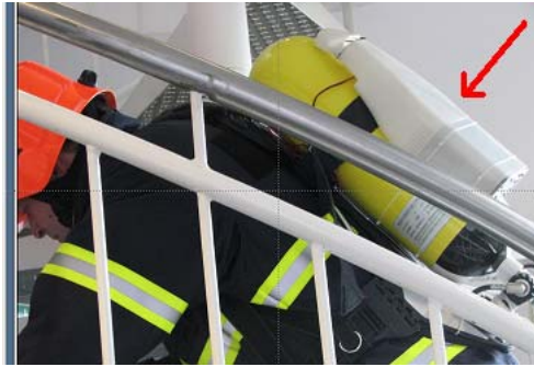
Fig. 1. Prototype of sensor dispenser for automated hands-free node deployment. Photo: BIBA, Germany.
