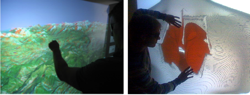
Fig. 5. Two examples of applications interfaced by the iMUTS interaction paradigms. (Left) a user interacts in a landscape-planning scenario on an FTIR multi-touch wall with an anaglyph-based stereoscopic projection. (Right) a user performs volume deformation in a medical scenario using a large FTIR-based passive back projection iMUTS.
