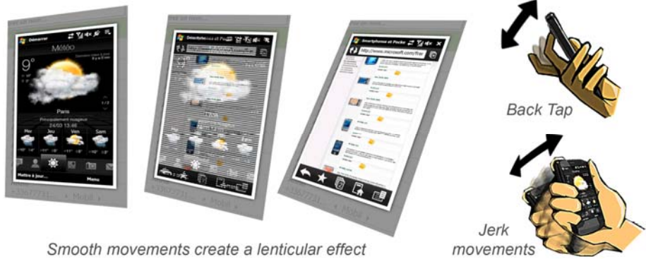
Fig. 1. TimeTilt helps to "travel in time" to reach previously opened windows. A tap on the back of the device triggers a continuous mode so that the user can navigate through windows by performing smooth gestures. A discrete mode can be activated with jerk movements.
