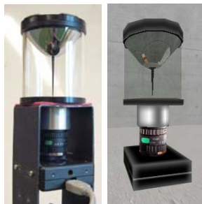
Fig. 1. The catadioptric omnidirectional camera, real and simulated
