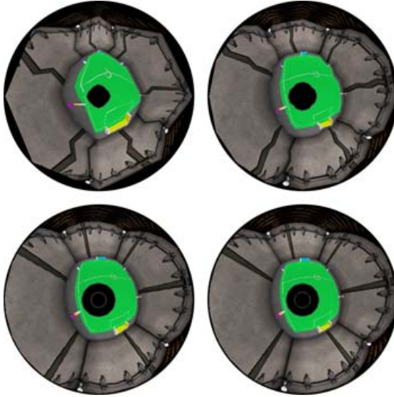
Fig. 8. 360 \times 360 Pixel mirror surface view comparison. Top left: 16 polygons. Top right: 64 polygons. Bottom left: 256 polygons. Bottom right: 1024 polygons.
