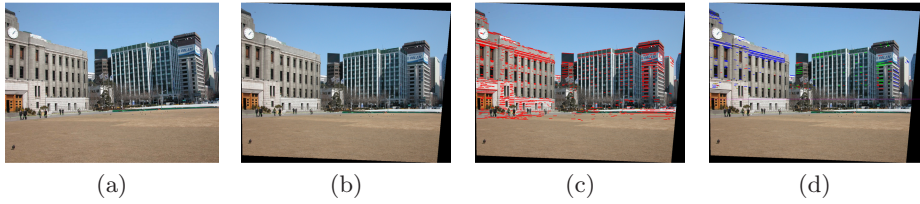
Fig. 3. Preprocessing scheme (a) Source image (b) Tilt corrected image (c) Extracted lines after filtering (d) Horizon estimation and vanishing point estimation. Lines, which refer to the same vanishing point, are shown with the same colors
