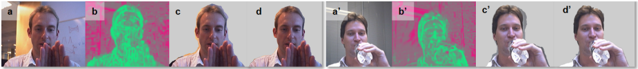
Fig. 8. Segmentation results in the presence of weak, stereo unaries. (a, a') Frames from two stereo videos. (b, b') Stereo likelihoods, with large uncertain areas (in grey). (c, c') GeoS segmentation, with no contrast sensitivity. (d, d') As in (c, c') but with contrast sensitivity. Now the segmentation accurately follows the person's outline.
