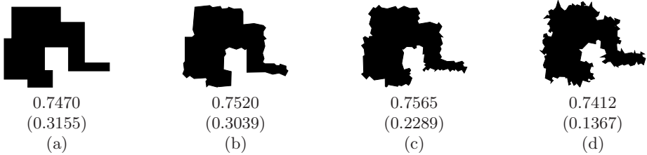
Fig. 4. Measured circularity \mathcal{C}(S) of a shape with added noise. Measured \mathcal{C}_{st}(S) circularities are in brackets.
