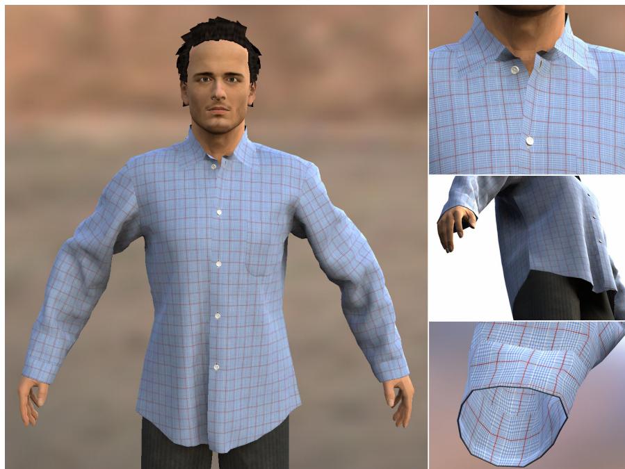
Fig. 2. An avatar dressed with a shirt. The close-ups show details like the collar, the 3D buttons and seam threads. The image in the lower right was rendered without the avatar and self-shadowing to visualize the cloth thickness and the seam allowance of the cuff.
