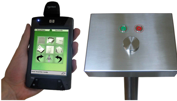
Fig. 3. PDA (3D interaction mask) and an interaction device with knob and buttons
