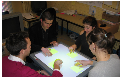
Fig. 1. Example of a tabletop system using MERL DiamondTouch device [5]
