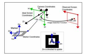
Fig. 3. Coordinate system used in AR ToolKit
