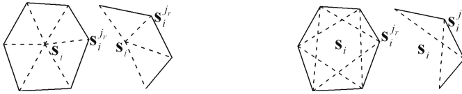
a) Stretching springs for case 1) and 2) b) Bending springs for case 1) and 2)
