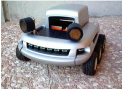
Fig. 2. K-Team's Koala robot equipped with a ring of 16 infrared sensors. The proposed technique is applied to the readings obtained with the highlighted frontal sensor
