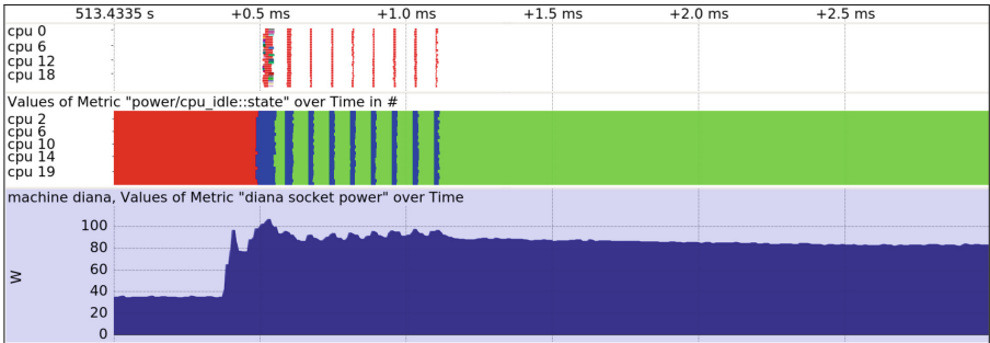
(a) Repeatedly sleeping for short intervals causing an idle time misprediction. Top: scheduled tasks per CPU, middle: core C-state requested by the menu governor (active [blue], C1E [green], C6 [red]), bottom: power consumption. Note that only socket power measurements are available at this time granularity.
