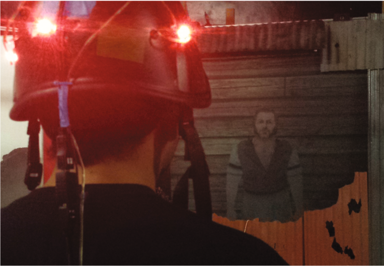
Fig. 1. An over-the-shoulder view of a user interacting with a virtual human, presented with REFLCT, a near axis, head mounted, retro-reflective projection display. The character and wooden wall pattern are projected. The corrugated materials are real props mounted around the retro-reflective screen.
