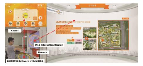
**Fig. 4.** A scene from interacting with SMARTIS (virtual apartment previewing system) using natural gestures, finger tracking, touch, multiple displays and voice commands.
