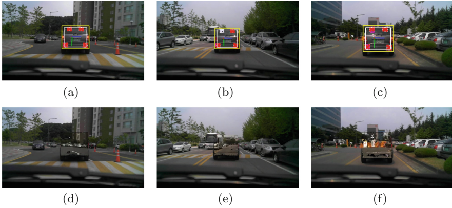
Fig. 8. Real time results in real condition, (first row) markers detection and pose estimation, (second row) Seeing-through results
