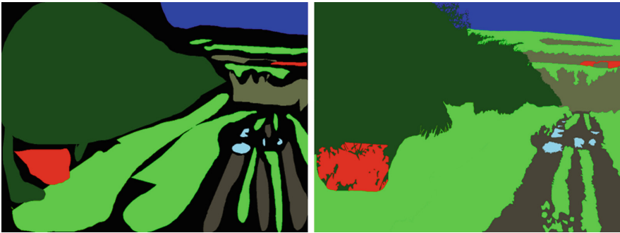
Fig. 4. Partial and fully labelled versions of the same image from our off-road data set. Fully manually annotating an image like this can take a person several hours, while a partially annotated image can be created in a few minutes. In our partially labelled training set, 69 % of pixels are labelled
