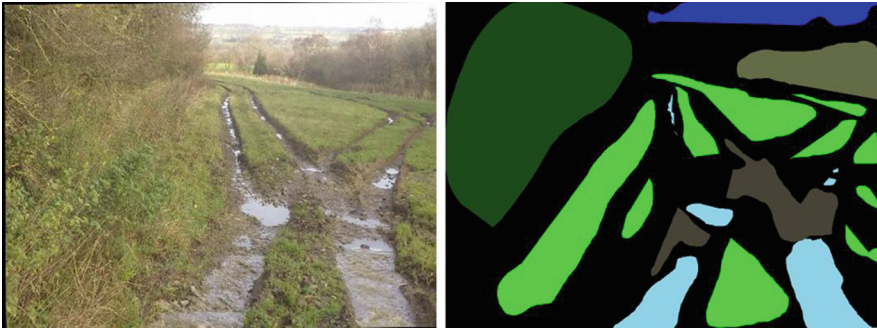
Fig. 3. An example image from our off-road dataset next to its partially labelled training image
